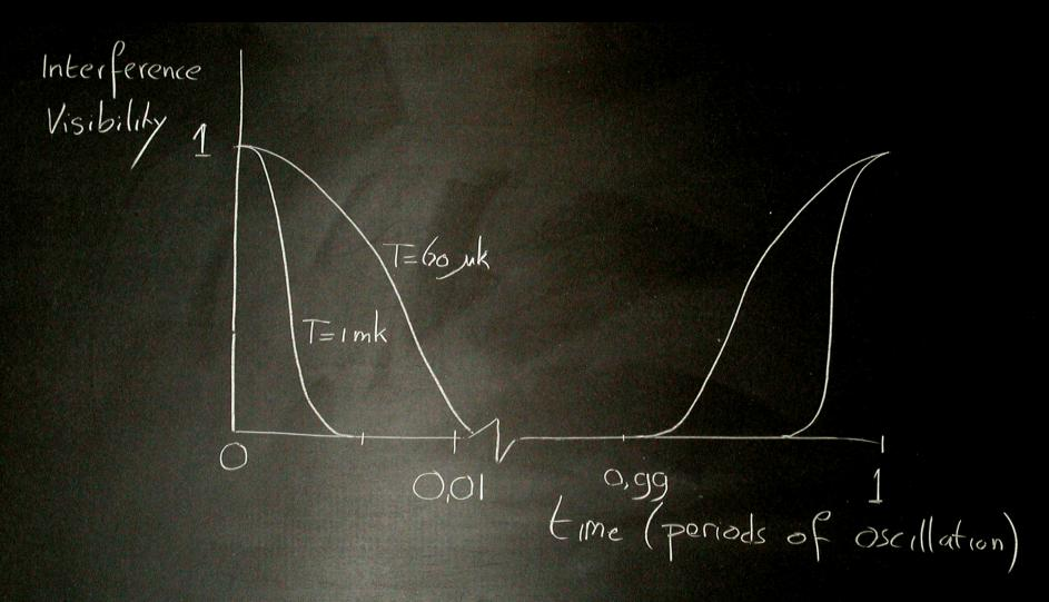
T is effective temperature of the fundamental resonance of cantilever
