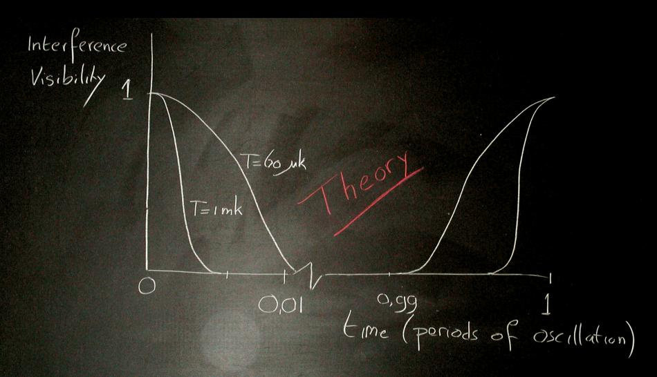
T is effective temperature of fundamental resonance of cantilever
